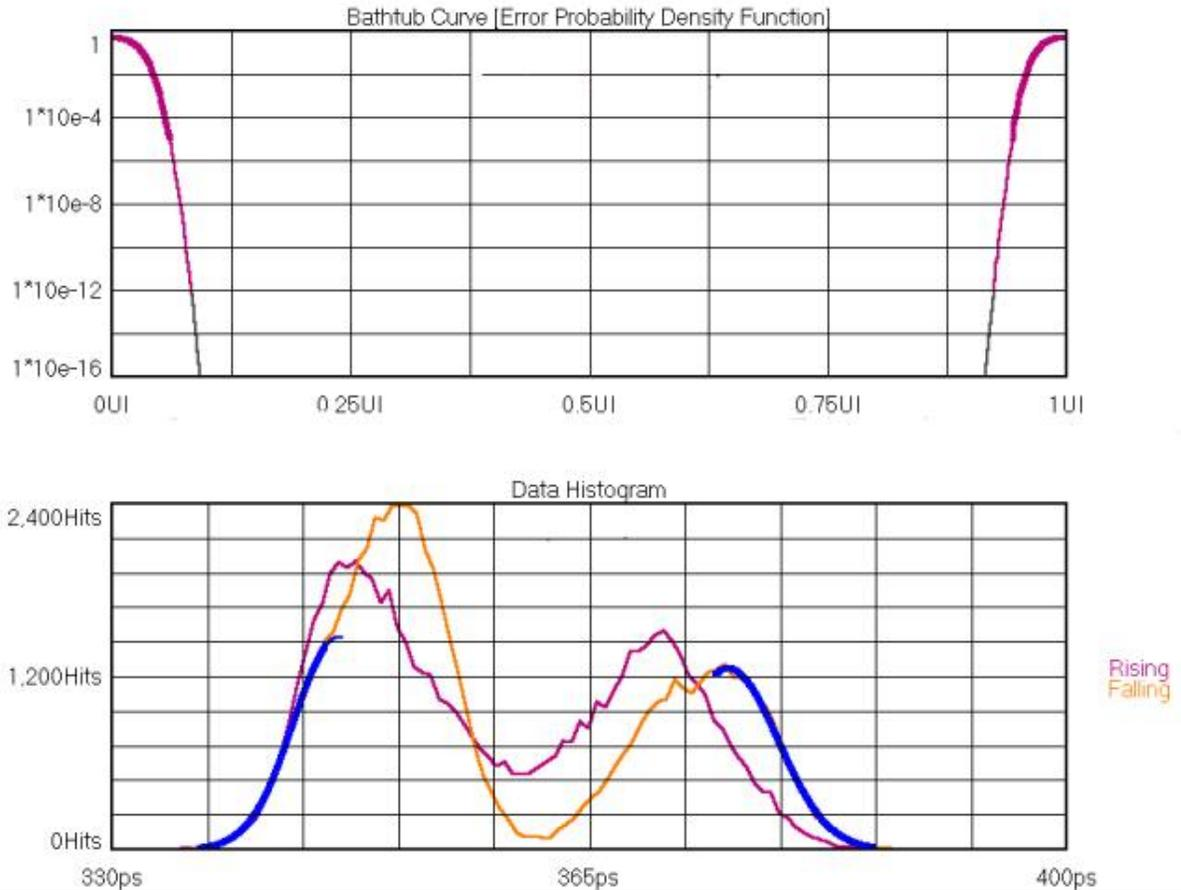
**Figure 9.** Typical data acquired with a TIA using clock-to-data method. Bottom figure shows histograms for rising and falling data edges. This view enables the user to determine the jitter contribution from the polarity of edges. The right and left most portion of the histograms are fitted with Gaussian tails in order to determine the  $1\sigma$  for RJ, the difference between the means of the Gaussian distributions is the DJ value. The top figure shows the bathtub curve.
