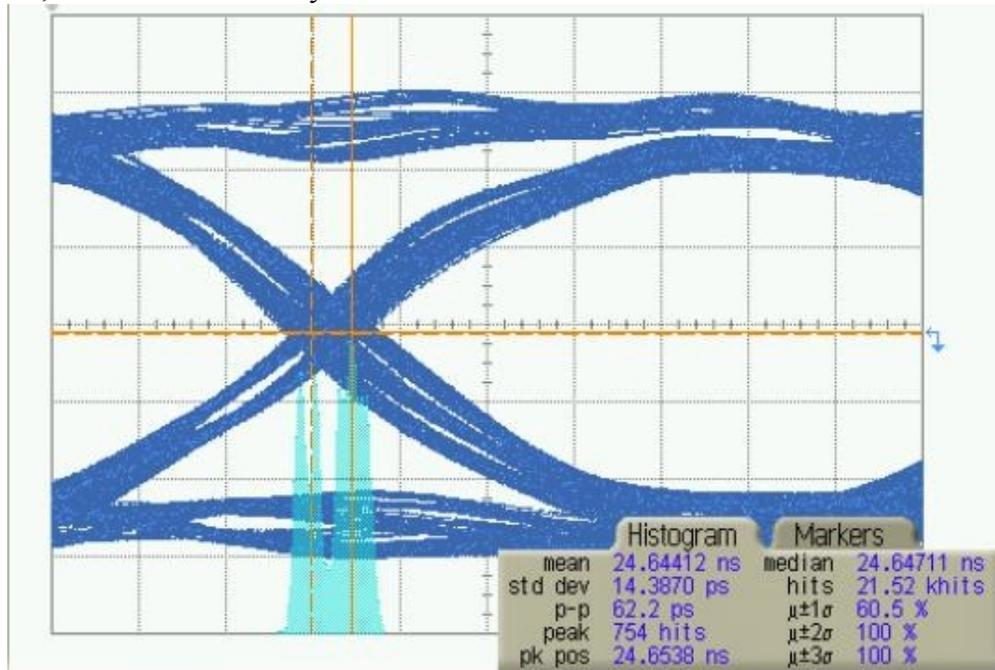
**Figure 7.** Output from an oscilloscope showing the data crossing points and the resultant histogram acquired at the crossing point. In this example the pk-pk value is 62.2 ps for a histogram with 21,520 hits was acquired over a  $\sim 3$  minute time period.
