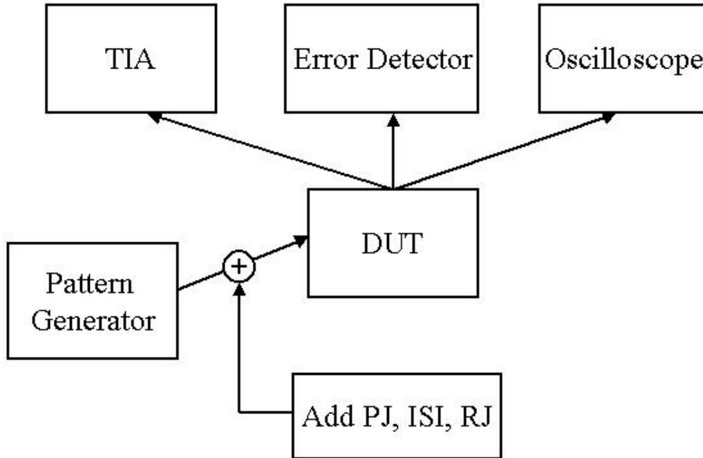
**Figure 11.** The experimental setup consisted of a pattern generator that transmitted a pattern to the Device Under Test (DUT). PJ, ISI and RJ could be added to the transmitted signal. The pattern was then input to the DUT and then output to the Error Detector, Oscilloscope or TIA for jitter analysis.
