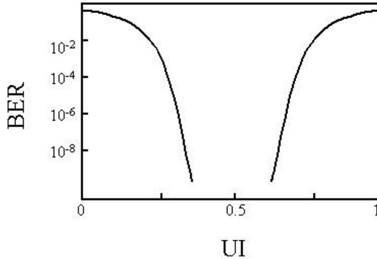
**Figure 8.** A bathtub curve showing BER as a function of eye closure.
