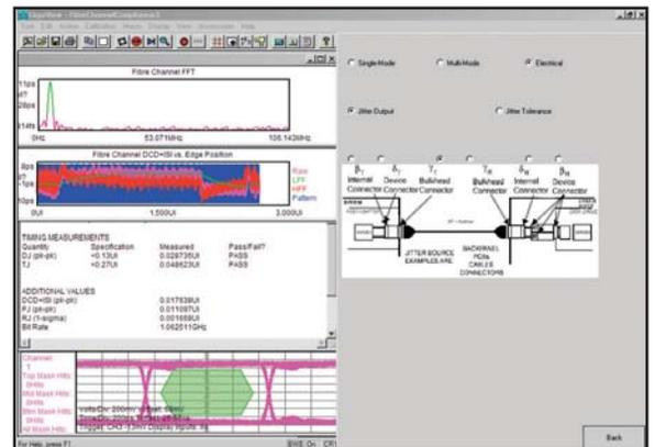
Perform compliance and mask testing, pass/fail for 1X Fibre Channel and other applications
