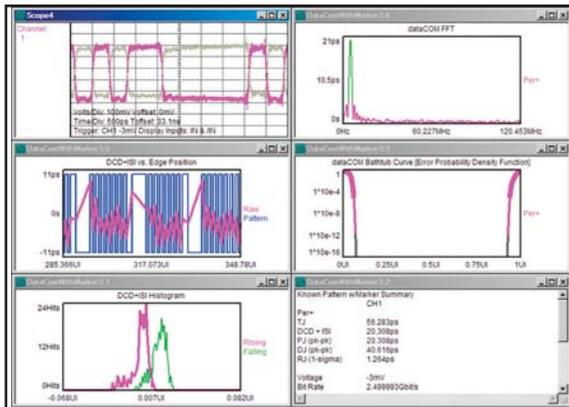
Diagnose serial data RJ, DJ, TJ, jitter spectrum, etc.
