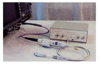
Setup showing the active differential probe solution. Picture at left shows Agilent part numbers; 1134A, E2675A, N1022A, 1143A and WAVECREST part number 030604-00.
